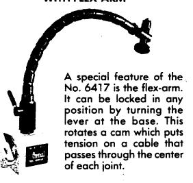
If the arm will not lock in position, adjust cable length by turning the knurled nut, located under the cross head, at the outer end of the arm.
